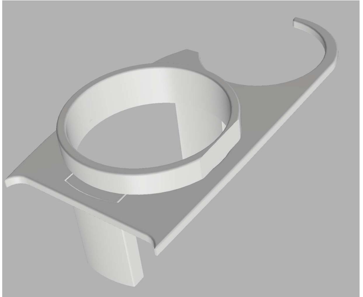
The cupholder is manufactured via 3D printing. The product will be sufficiently strong for this purpose, but low volumes means a more fragile product when disassembled and assembled again.
